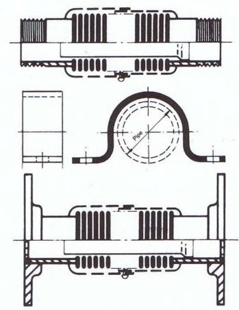
For steel and copper pipes sizes 15 mm to 150 mm LPHW, MPHW, HPHW, STEAM AND CONDENSATE, SECONDARY AND PRIMARY HWS. Tube guides are particularly suitable in vertical service risers where space is of prime importance in high rise buildings. The installer must slide the guide over the pipe before welding on flanges. Mounting feet can be turned through 90° for fixing to a single channel or alternatively, flat plates for bolting to channel face.
