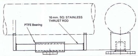
MULTI-SERVICE APPLICATIONS FOR WELDING DIRECT TO THE PIPEWORK. CAN ALSO BE FITTED WITH IH 100 PIPE CLIPS FOR BOLTING TO THE PIPEWORK.
