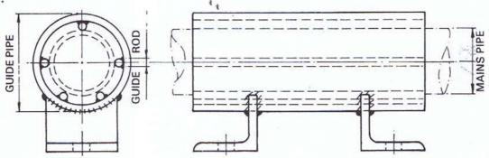
PIPE SLIDE GUIDE 1H 184 (Suitable for pipes up to 80mm)
