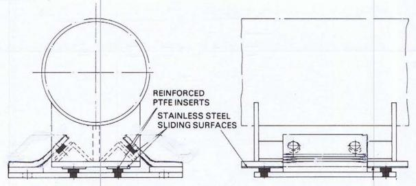
HEAVY SLIDE GUIDE IH 189C For welding direct to the pipework application as per 189 A guide
